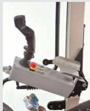
ERO Comfort Controller with joystick operation
