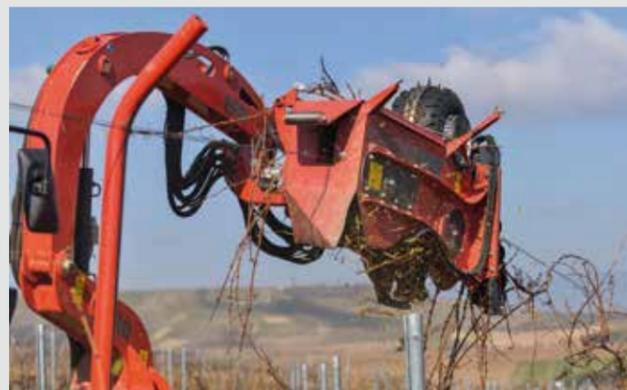
Cane Pruner VITECO working head with hydraulic adjustment on two axes
