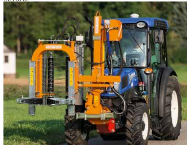
Adjusting to a different cutting length takes very little time. The VSL07 P is therefore just as suitable for cordon-trained as for cane-pruned vines. Its low weight makes the VSL07 P suitable also for use on steep slopes and in difficult terrain.
